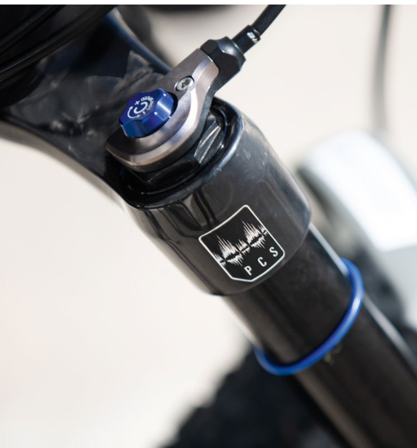
NLO Hydraulic Lockout with fixed rebound damping.
