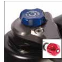
RL-RC Remote speed Lock out Rebound adjust Low speed Compression adjust
