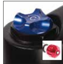
RC Rebound adjust Low speed Compression adjust
